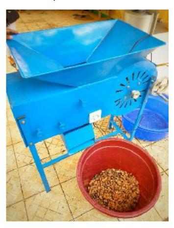
In preparation for the big nutmeg harvest season in October to January, GEG has procured two types of agricultural machines: one to automate the process of separating the nutmeg from its shell (huller) and the other to separate the nutmeg from its husk (blower). This initiative is carried out to increase the efficiency of the post-harvest processes which hopefully will bring a positive impact to the quantity and quality of the nutmeg produced.
